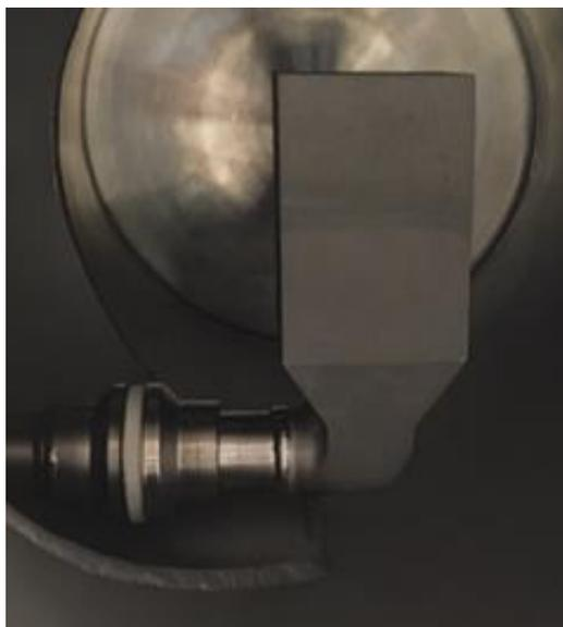
**Figure 2.11:** Image of the titanium blocker positioned in the beam line end station for irradiation. The beam enters normal to the front face.
