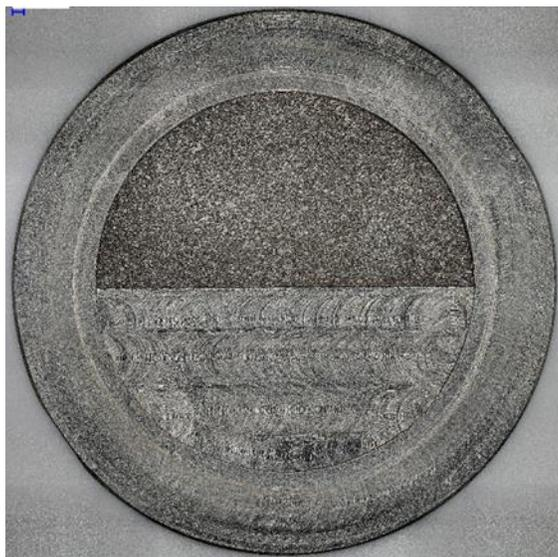
**Figure 2.4:** Optical image of the irradiated Ti64 disk. In this image, the top half of the disk was left as the rough 3D-printed material and the bottom half was milled smooth.
